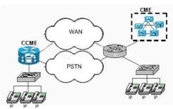
Refer to the VoIP network shown in the exhibit. On which link in the network would the QoS mechanism Compressed Real-Time Transport Protocol (cRTP) most likely be deployed?
