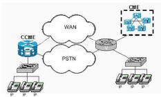
Refer to the VoIP network shown in the exhibit. On which link in the network would the QoS mechanism link fragmentation and interleaving (LFI) most likely be deployed?
