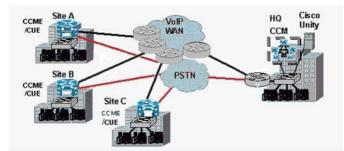
In the network shown in the exhibit, VoIP is used over the intranet WAN to facilicate all voice communications between all sites. Calls out of the intranet are made direct via the PSTN at each site. Choose the two appropriate network devices upon which AutoQoS should be implemented to facilitate proper voice quality for inter-site calls. (Choose two)
